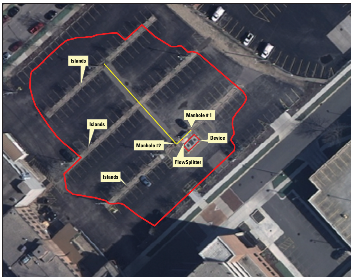
Figure 1. Study area including the drainage area of the parking lot (outlined in red), and location of the islands, manholes, and flow-splitter box and storm-sewer pipes (lined in yellow).
